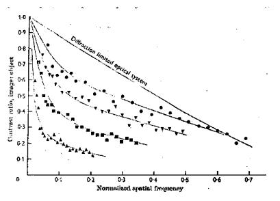
In this figure, the estimated MTFs are plotted for various pupil sizes (2, 2.8, 3.8, and 5.8 mm). The curves are normalized so that the diffraction limit would correspond to a frequency of 1. The solid line is the diffraction limit. You can see that for high frequencies, the eye with a 2mm pupil is essentially diffraction limited. However, aberrations (e.g. spherical) greatly affect contrast for big pupils.
